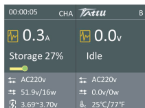
a) Single battery charging storage interface
